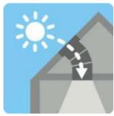
The **rigid** tunnel is ideal for distances between roof and ceiling from 0.9 to 1.7 m - with extension sections up to 6 m.
